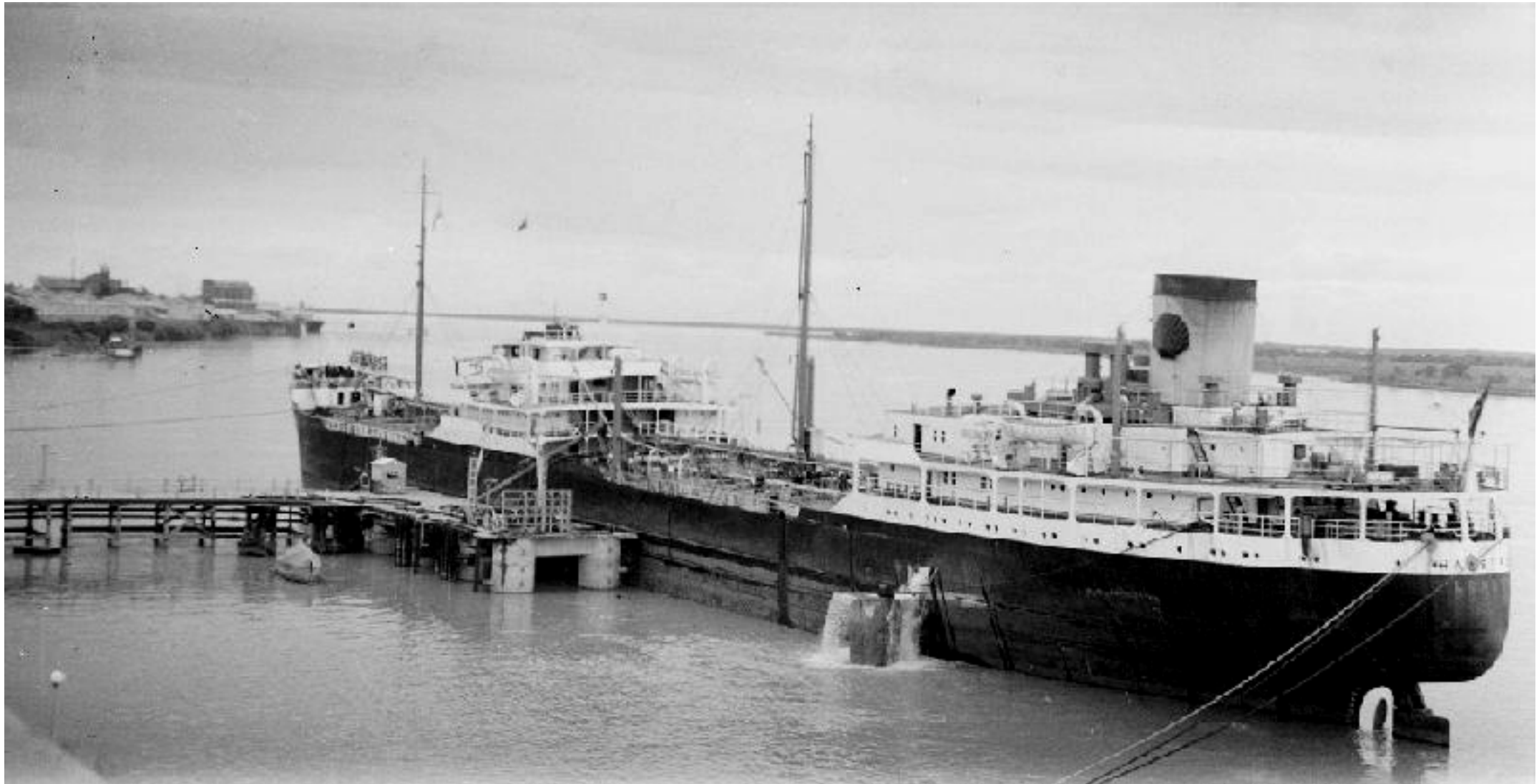
Haustrum built Hawthorn, Leslie & Co, Hebburn on Tyne February 1954 12090 G tons, Steam Turbine. Scrapped in Taiwan July 1975
